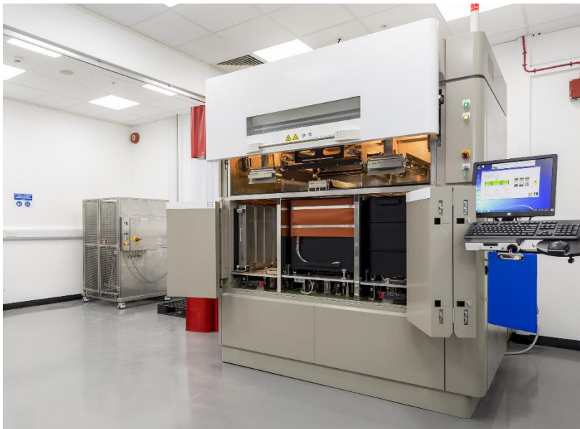
High-end Additive Manufacturing technology: The RICOH AM S5500P
