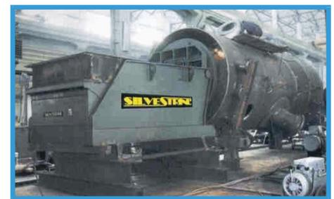
**Positioners type AVSA - with capacity from 0,1 to 40 ton., are provided with a third movement, besides rotation and tilting, the lifting.**
