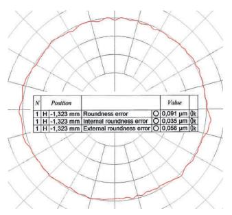
The chart shows a run-out of the main spindle of 0.09  $\mu m$  at 3,200 rpm. This run-out accuracy was measured on a 17 year old Super-Mikroturn®. The Mikroturn® machines have an everlasting accuracy due to the absence of metal contact between the moving parts.
