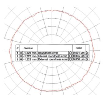
The chart shows a run-out of the main spindle of 0.09  $\mu m$  at 3,200 rpm. This run-out accuracy was measured on a 17 year old Super-Mikroturn®. The Mikroturn® machines have an everlasting accuracy due to the absence of metal contact between the moving parts.
