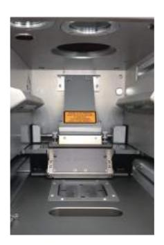
In addition, the SLM 125 provides a **build volume reduction** of  $50 \times 50 \times 50 \text{ mm}^3$  thus decreasing the amount of powder by 80%
