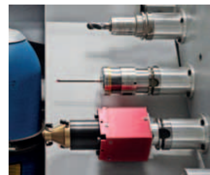
Tool, measuring probe and fibre laser unit in the tool changer
