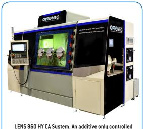
LENS 860 HY CA System. An additive only controlled atmosphere model. LENS 860 AM CA is also available.
