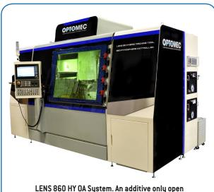
LENS 860 HY OA System. An additive only open atmosphere model, LENS 860 AM OA, is also available.
