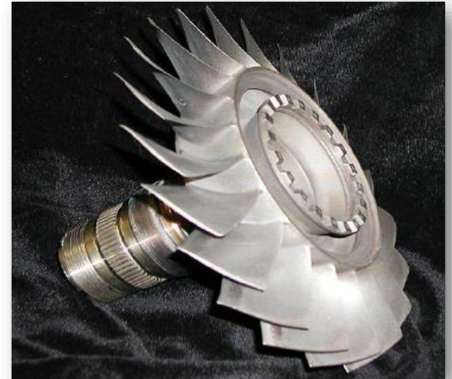
After finishing and successful spin tests
