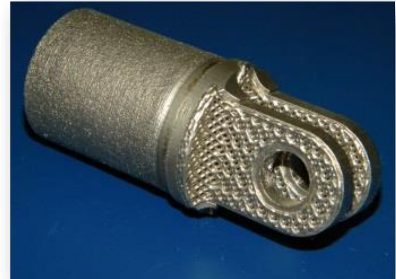
LENS used to extend shaft length on PBF fabricated fork joint
