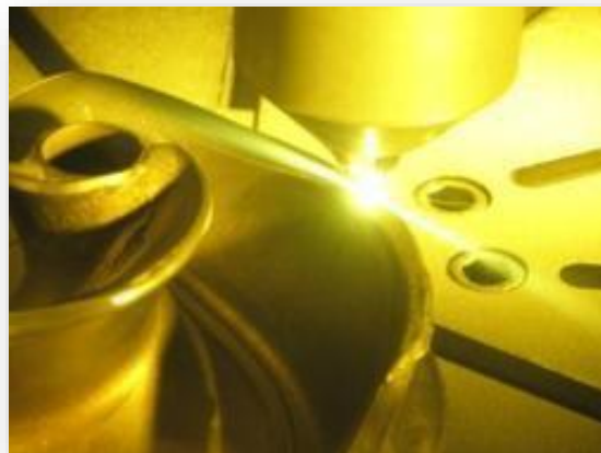
Using LENS to restore worn areas
