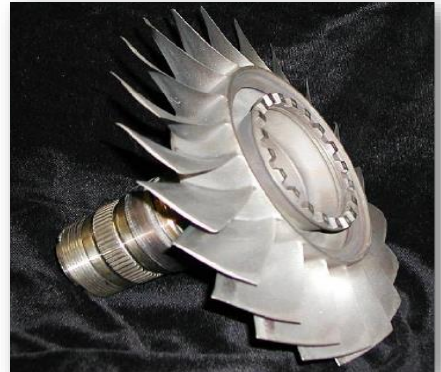
After finishing and successful spin tests
