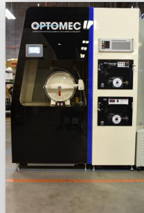
500 W and 1 kW lasers are rack mounted. This side view of the LENS 860 shows a 1 kW laser (top right, above 2 chillers).
