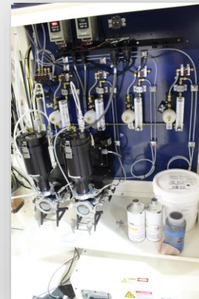
Side view of LENS 860 shows 2 powder feeders mounted to the side panel. A total of 4 powder feeders can be mounted.
