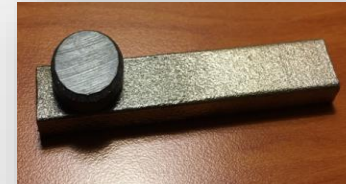
Functional grading- the bar was printed starting with carbon steel (magnetic) then transitioning layer by layer to stainless steel (non-magnetic).
