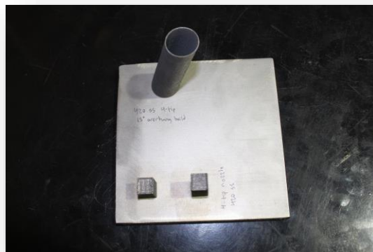
15deg overhang build and cubes- 420 SS, 4-tip nozzle
