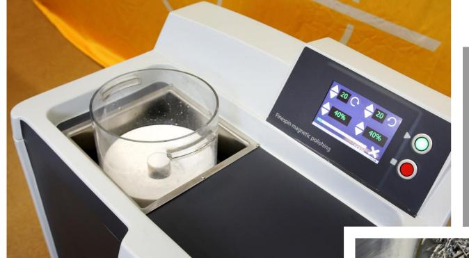
The container is placed on top of a rotating magnet plate.
