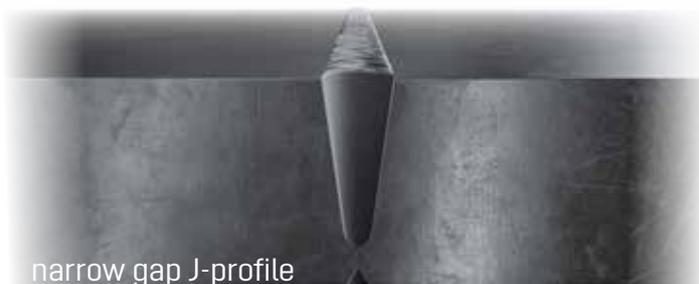
The reduction of welding joint volume minimizes the costs of consumables and increases production speed.
