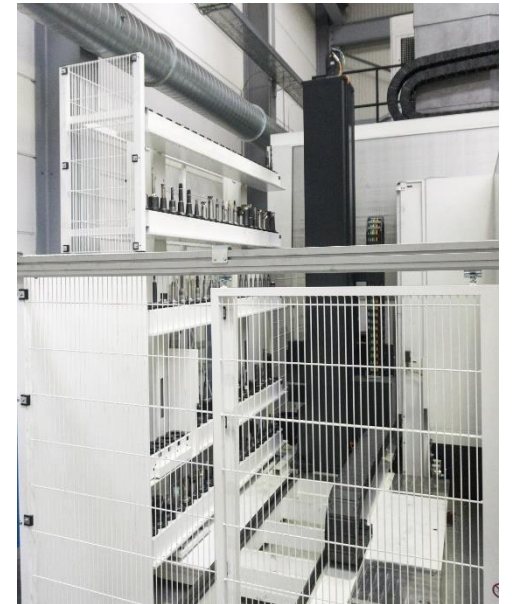
Fully automated tool magazine with 100 pockets for automatic change into all spindle units
