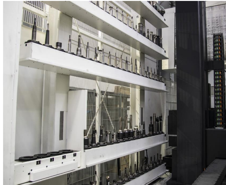
Fully automated tool magazine with 100 pockets for automatic change into all spindle units
