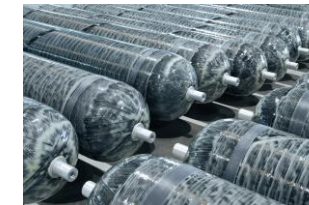
Hydrogen pressure vessels
