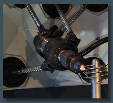
wire-based laser system with 2kW
