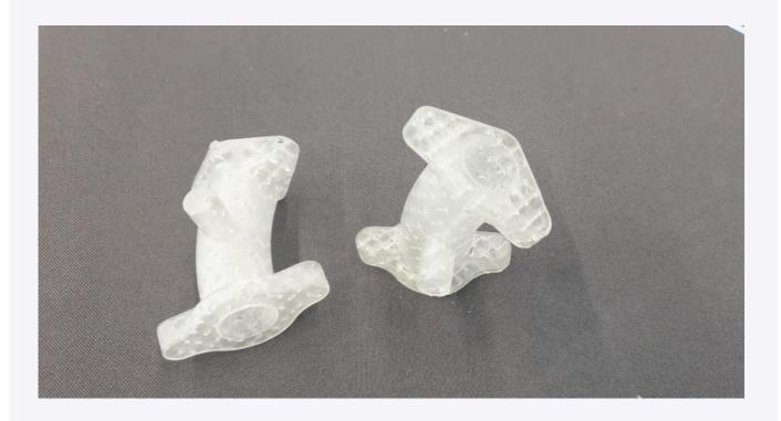
RR355-101-CAS is a Direct casting material that was formulated for our Raplas production equipment. RR355-101-CAS offers the best performance characteristics as follows: low deformation due to shrink, strength, durability, water resistance. The RR355-101-CAS is transparent in colour.
