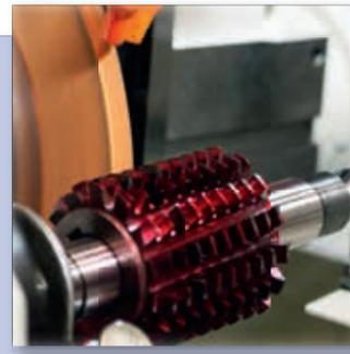
Cylindrical and angular infeed grinding
