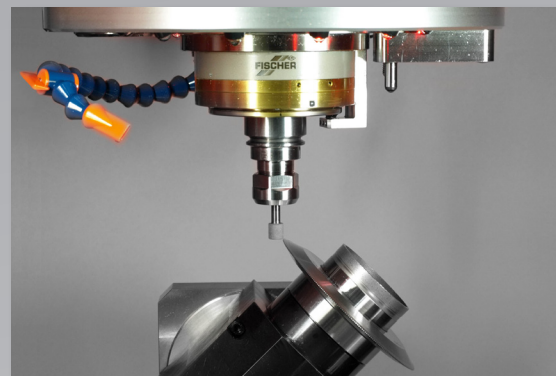
Automated dressing in optional jig grinding package
