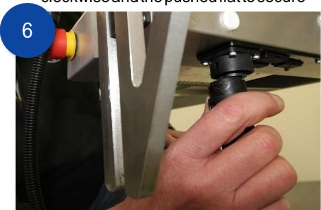
Connect the *X Beam Upper* cable into the *X Beam Lower* socket
