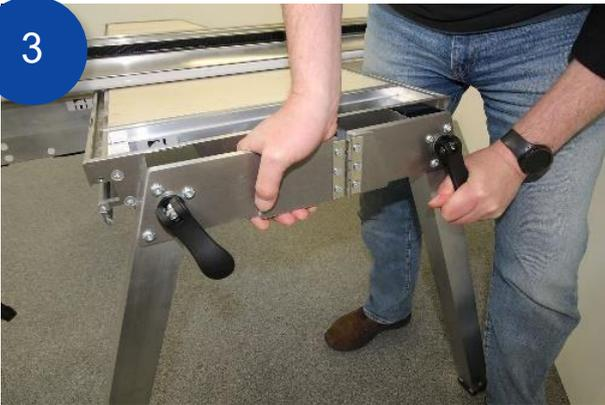
Push the clamp handles down flat to the *Y Bench* end plate to tighten.
