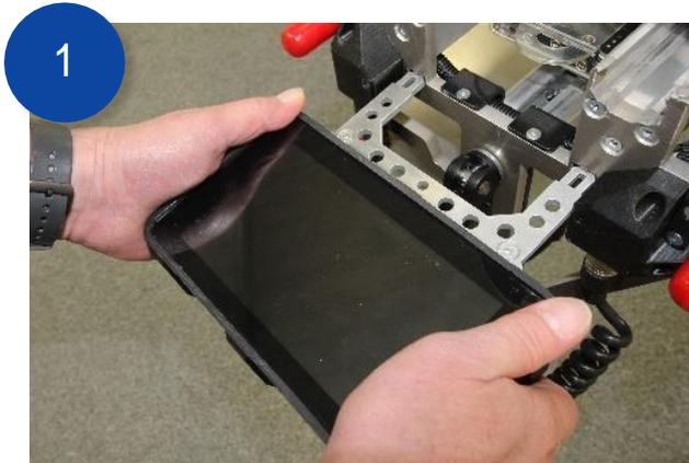
Place the *Console* into the locating slots in the E Stop end of the X Beam Upper.
