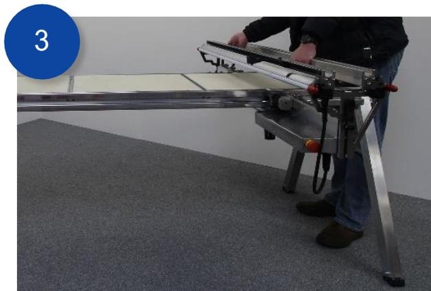
Slide the *X Beam Upper* down until the rollers rest on the *Y Bench*
