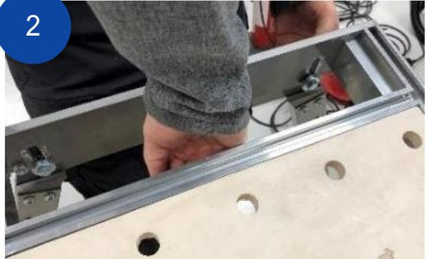
Slide the leg clamp pins into the slots in the *Y Bench* end plate.
