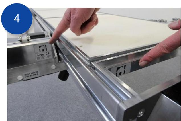
4 Slide the *X Beam Lower* onto the *Y Bench* such that both Home Icons face the same way, as shown.
