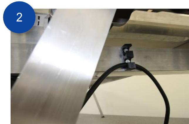
Hook the mains *power cable* over the strain relieving bracket to ensure it doesn't unplug during operation.
