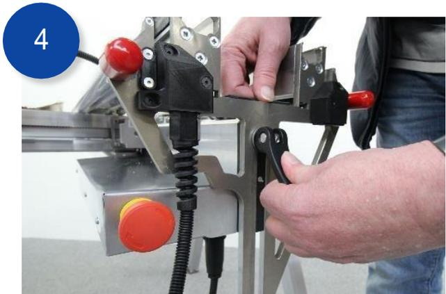
The quick release handle can now be rotated clockwise and the pushed flat to secure
