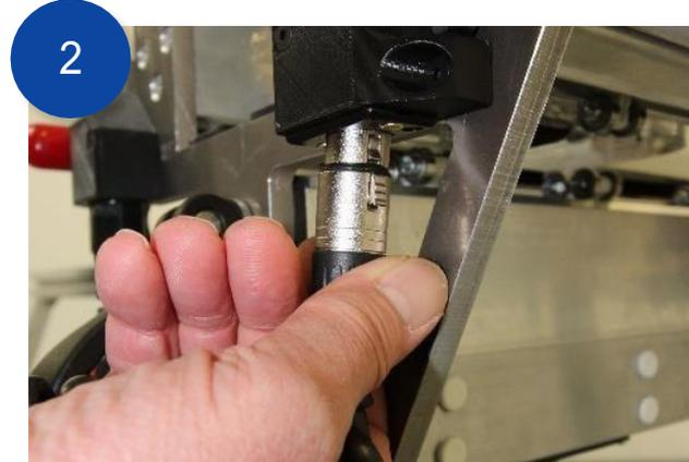
Plug the *Console* cable into the connector on the right-hand side of the X Beam Upper.
