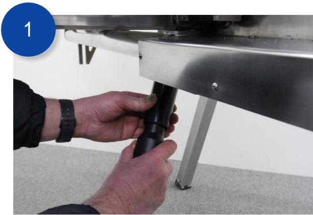
1 Attach the extraction hose to the underside of the *X Beam Lower*
