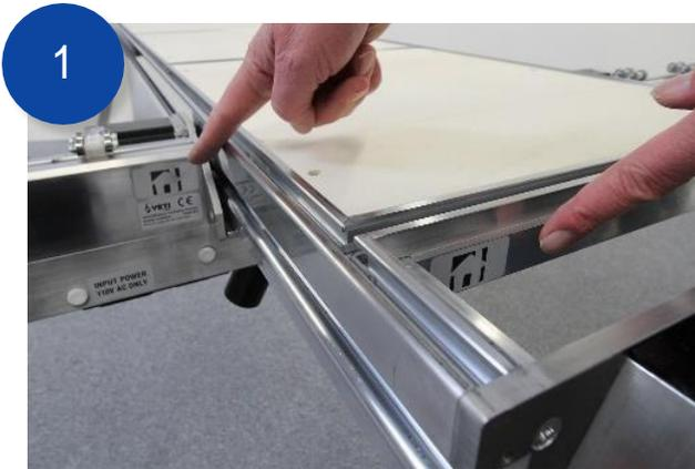
Identify on the Home Icon on the inside rail of the *X Beam Upper* (Figure 5, page 2). Position it above the *X Beam Lower*, so that all 3 Home Icons are visible from the same side.
