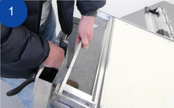
Unfold a *Leg Set* (Figure 3, page 2). Lift the *Y Bench* to accept the location pins of the *Leg Set*.
