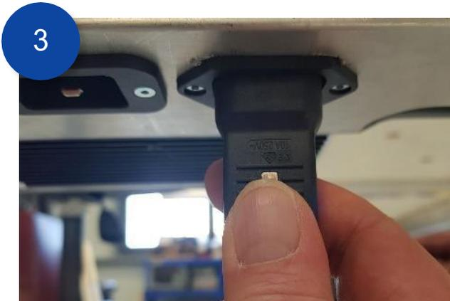
3 Or: if the extractor does not exceed the power rating, plug in your extractor to SmartBench's extractor power outlet
