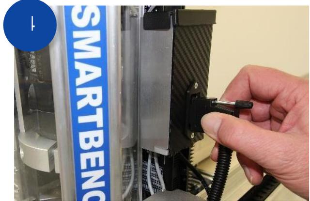
Connect the ZHead signal cable and secure using the thumb screw.
