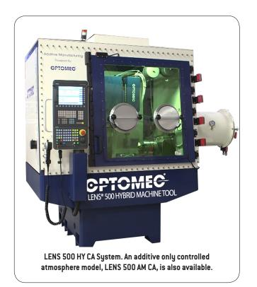
The LENS 500 Hybrid Controlled Atmosphere System sets a new standard in affordability and performance for titanium and aluminum metal additive manufacturing applications. The system incorporates an Optomec proprietary hermetically sealed Class 1 enclosure and an integrated gas purification system that maintains oxygen and moisture levels to below 40 ppm.
