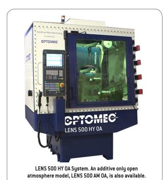
The LENS 500 Hybrid Open Atmosphere System sets a new price to performance standard for combining additive and subtractive manufacturing in a single machine tool. The system utilizes Optomec industry proven LENS Print Engine technology seamlessly integrated into Class 1 Laser Safe CNC platform. The system is ideally suited for processing stainless and tool steels, nickel-based alloys, cobalt, tungsten and other non-reactive metals.
