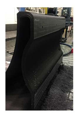
MasterPrint® Linear can **print**, **overprint** and **reinforce** hollow **structures** at any fixed angle between 0° and 90°.
