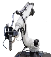
CARACOL: thermoplastic 3D printing on robots
