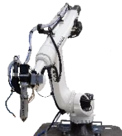
CARACOL: thermoplastic 3D printing on robots
