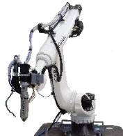
CARACOL: thermoplastic 3D printing on robots
