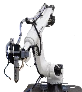
CARACOL: thermoplastic 3D printing on robots
