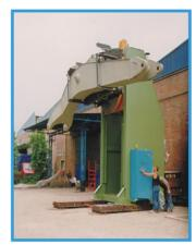
2. ELECTROMECHANICAL POSITIONERS WITH ROTATING TABLE for small capacities (from 50 to 3000 Kgs.) – Model SAE
