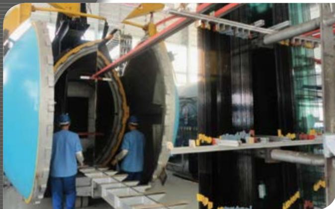
Panini manufactures autoclaves optimized for laminating of tempered or hardened glass in flat or curved formats. The specific process for PVB (polyvinyl butyral) ensures perfect bonding and transparency, without air bubbles or opacity. Our autoclaves are used in the following fields:
