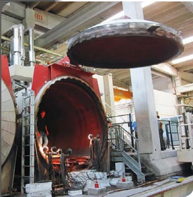
Panini offers autoclaves for heat and pressure treatment of stone and concrete, a growing segment of the construction industry with many uses, such as:
